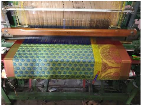
**Jacquard looms:** Jacquard looms are special looms that use punched cards to control the pattern of the fabric. The punched cards are fed into the loom, which uses them to determine which threads are lifted and which are lowered, creating intricate patterns.
