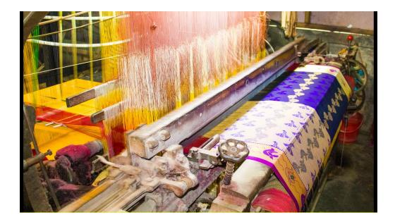
**Computerized looms:** CAD technology is used to design and create patterns for fabrics. The designs are created on a computer, and then the data is sent to the loom, which uses it to weave the fabric.
